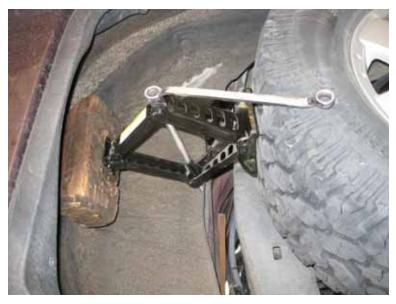
Each wheel you lift from gives you access to 2 body mounts eg. Front Drivers side you can get the front ds mount and t Back drivers side you can access the 3rd ds mount and the rear one.
