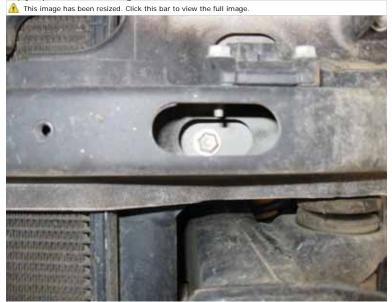
Tighten these support brackets and reinstall your fan shroud and overflowe bottle, and double check to make sure your radiator, or shroud.
