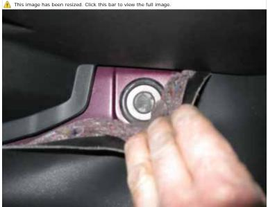
The last one is accessible from behind the cargo area trim. Remove your jack/tools cover and you will see the grommet passenger side is as easy as removing the inverter trim and it is behind that.
