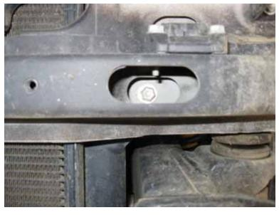
Slide the drop brackets in so the hex bolt goes through the rubber mount and the stud through the original support hol them, you may have interference issues with a nut located on the front bib panel. If you do, you can cut it off or install stop you plastic radiator hitting the nut.
