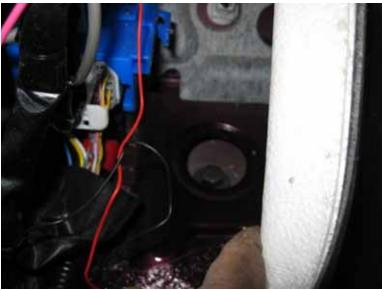
The 3rd one is next to the rear seat. Fold the base of the seat up against the fornt seats, and from where the child resti floor covering out from under the plastic side trim. The grommet and bolt hole wil be exposed in the corner of the floor.
