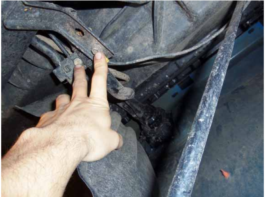
The cab bed bolts are T55 torx bit, an awfully strange bit for sure. I had to go to sears to pick up this bit as it is not a commonly used size.
