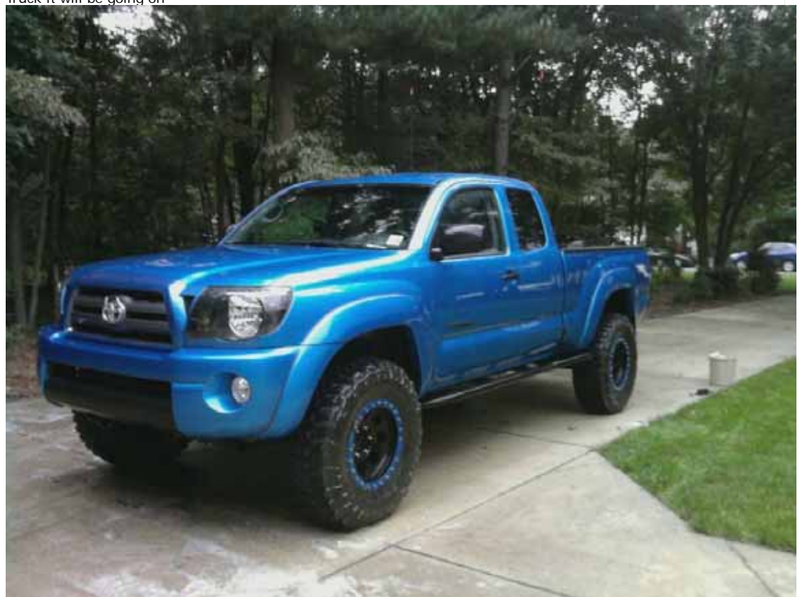
Before we start take some fender to ground measurements for the records Front, about 38"
