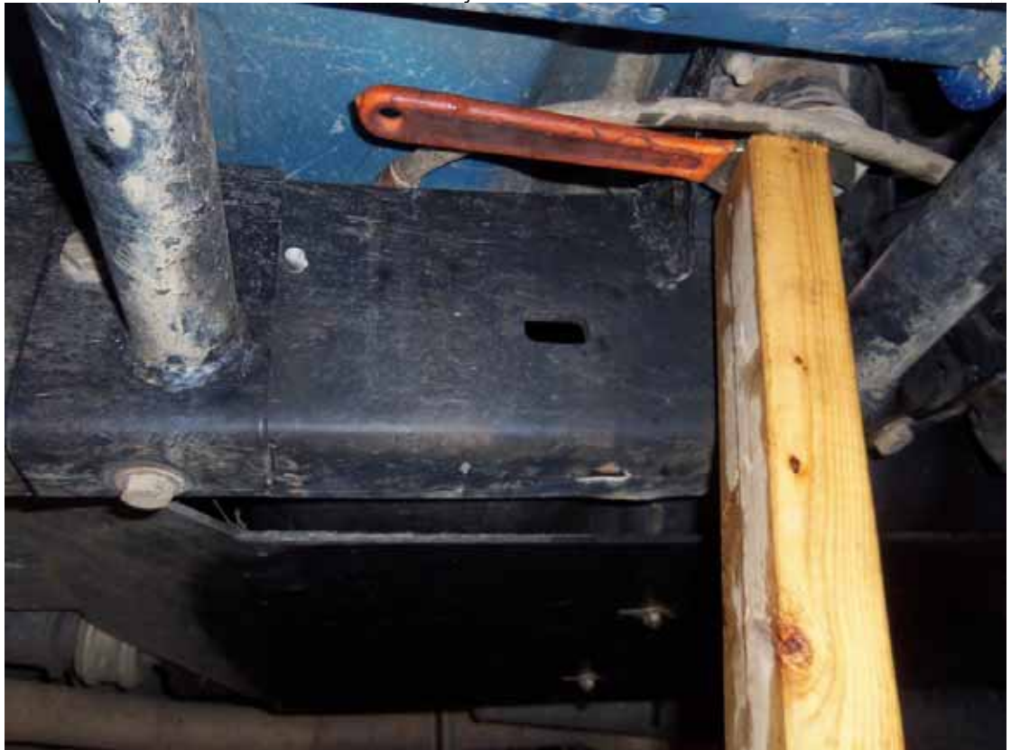
To hold the nut in place I used an adjustable wrench with a floor jack, this was a large metric nut and I did not have a deep well socket to fit it so the wrench worked just fine.
