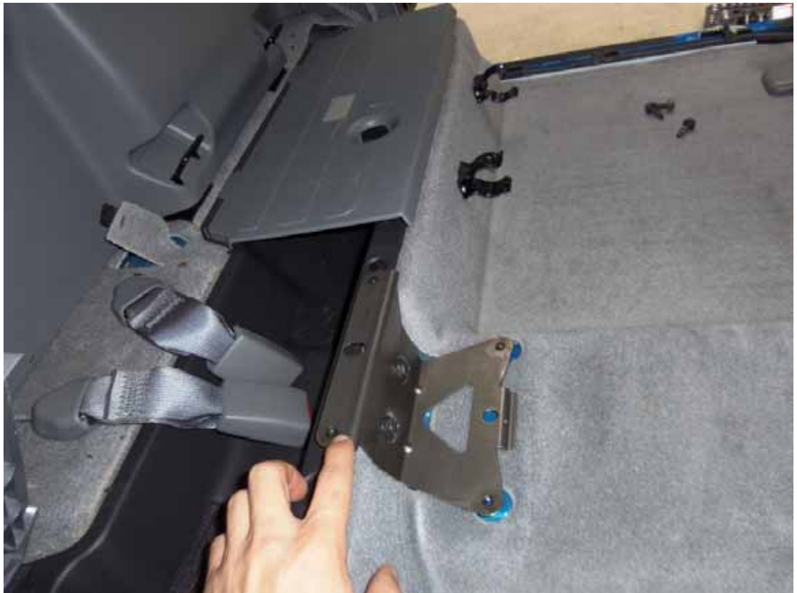
Remove the back seats, each seat is held in with 3 bolts all together, 12mm if I remember correctly. Peel back the carpet to access these bolts
