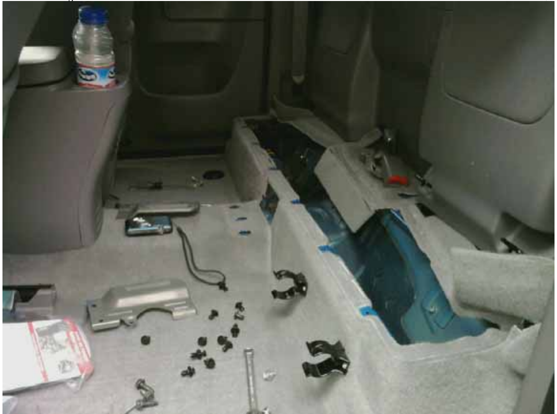
After all that is removed peel the carpet back a little more to access these small stiffening plates that are held in by two 10mm bolts, remove the bolts and plate
