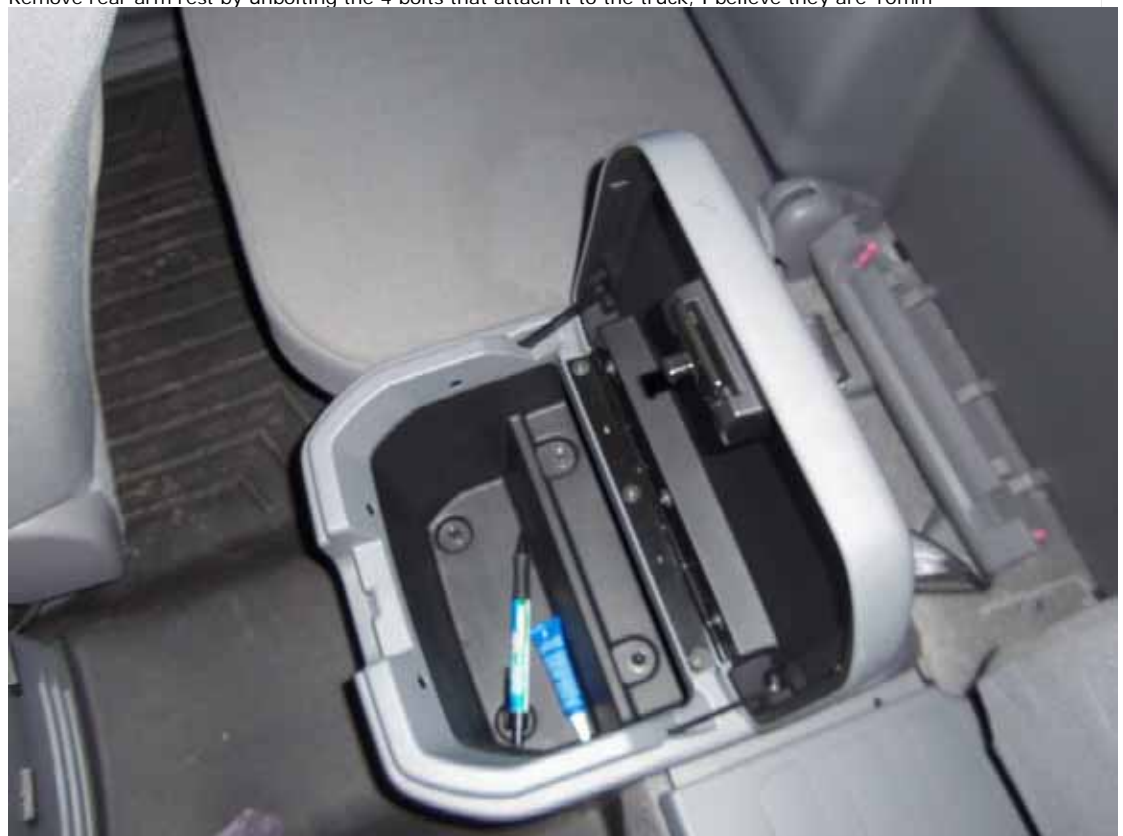
Once the arm rest is out of the way you can disconnect the bracket it bolts to, there are two 12mm bolts holding this on to the cab
