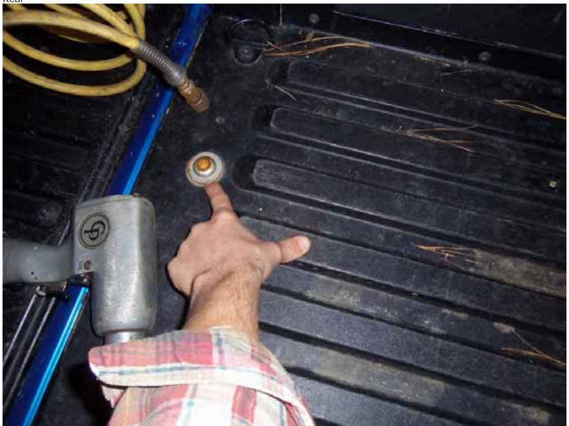
Where the bolt goes through the frame, through welded on captive nuts on the frame Front
