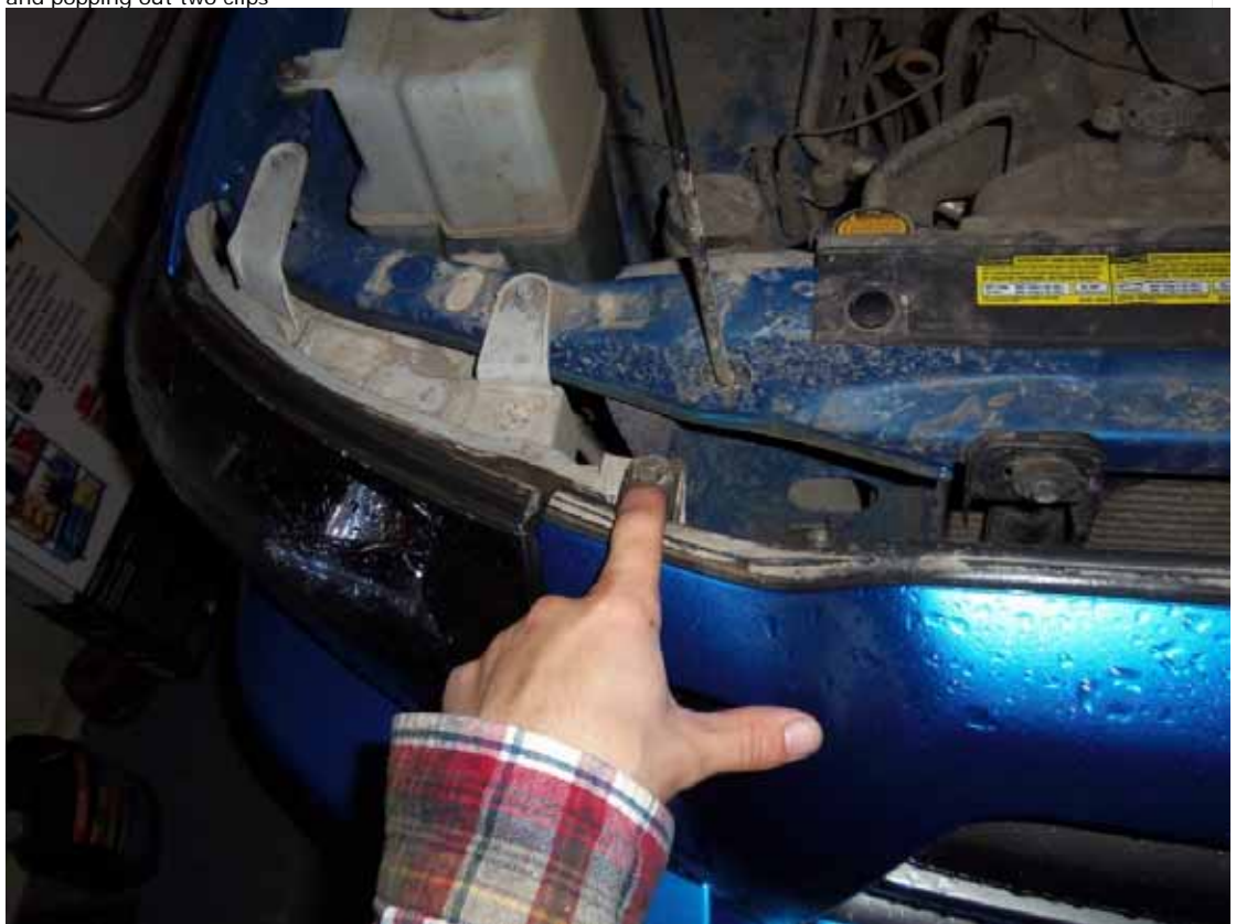
Give the grill a good yank upwards and it will unclip from the headlight assemblies, careful to use equal force on each side to not snap the cheap plastic Toyota tabs.
