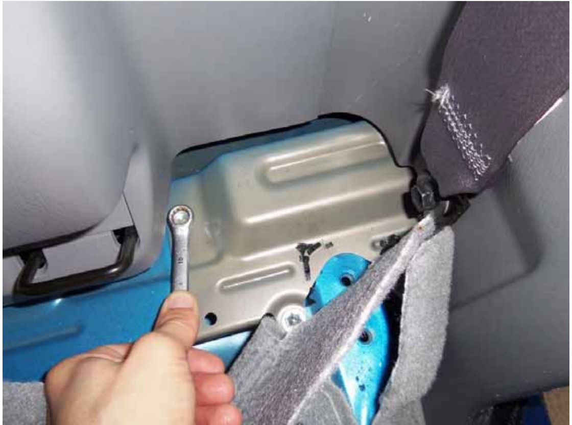
Below the plate there is another small plastic grommet, that is the access to the rear cab mount bolt, remove the grommet
