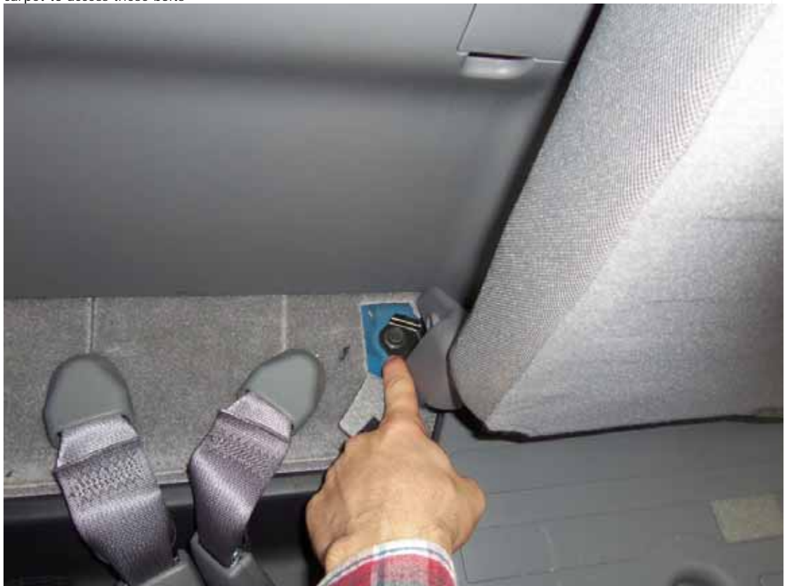
Remove the back seats, each seat is held in with 3 bolts all together, 12mm if I remember correctly. Peel back the carpet to access these bolts
