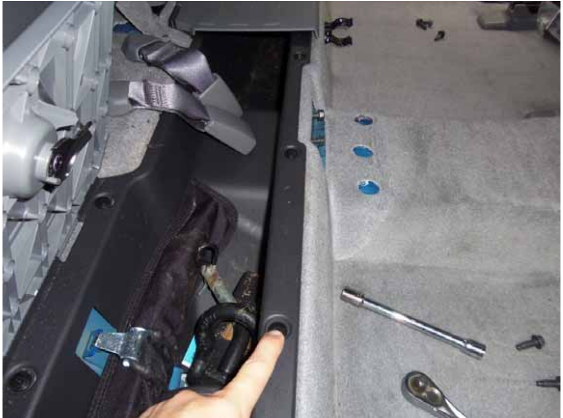
Once the lining is out it will look like this
