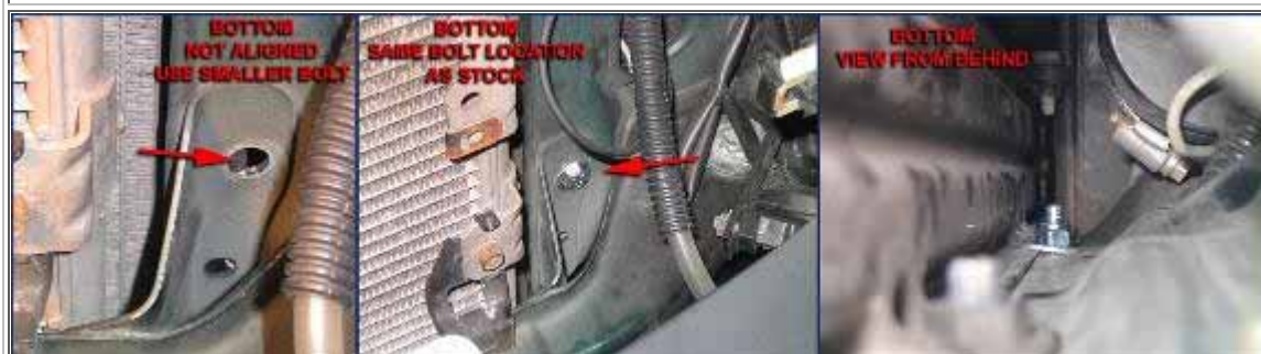
Radiator re-mounted 2" lower
