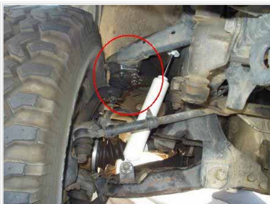
Ball Joint Spacer Installation
