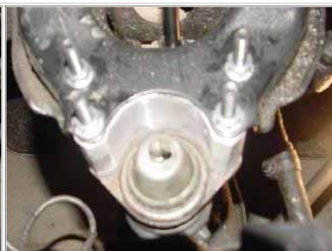
B: Spacer and Ball Joint Reinstalled
