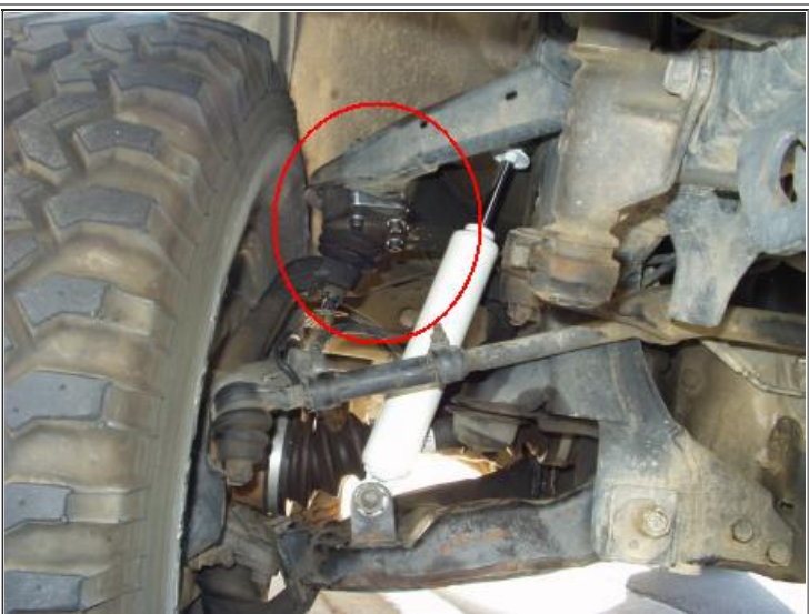
Ball Joint Spacer Installation
