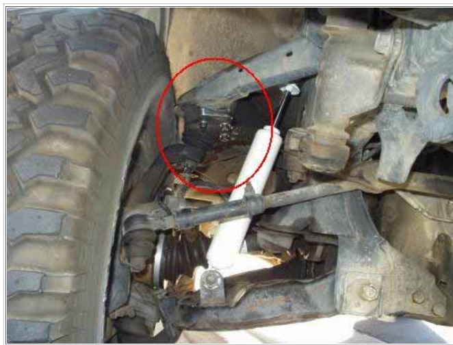
Ball Joint Spacer Installation
