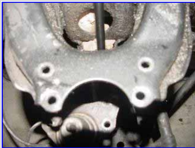
A: Upper Ball Joint removed
