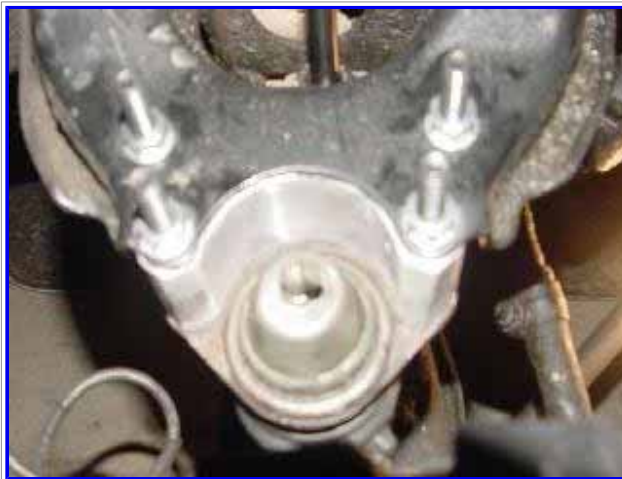
B: Spacer and Ball Joint Reinstalled
