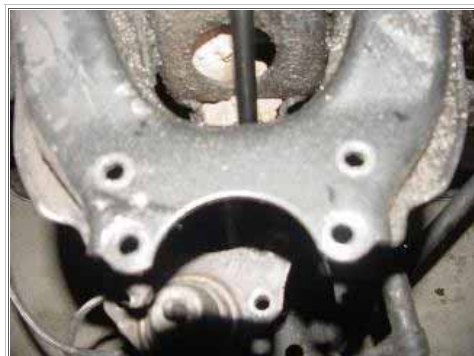
A: Upper Ball Joint removed
