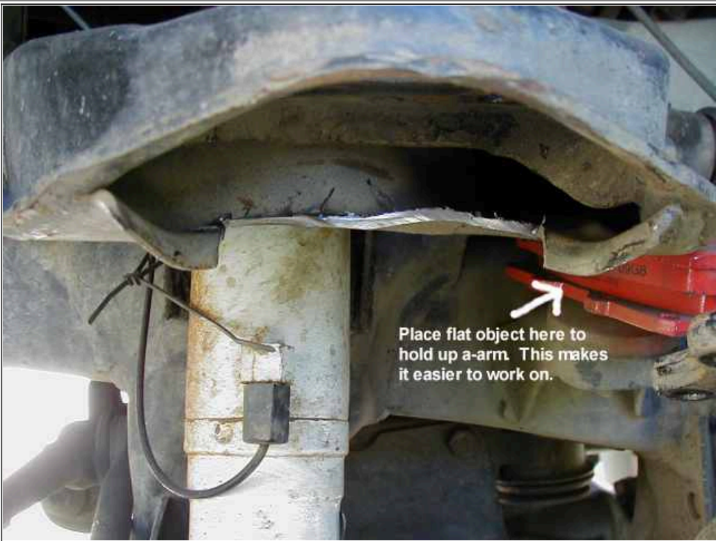
Trimming around upper ball joint
