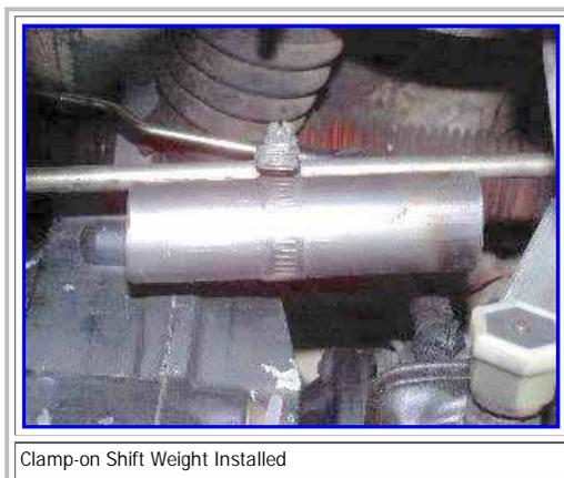
Clamp-on Shift Weight Installed
