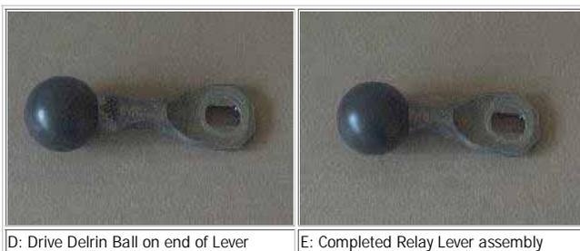
D: Drive Delrin Ball on end of Lever
