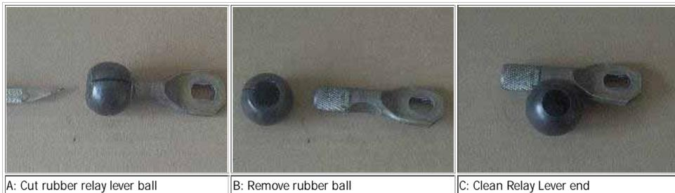
A: Cut rubber relay lever ball
