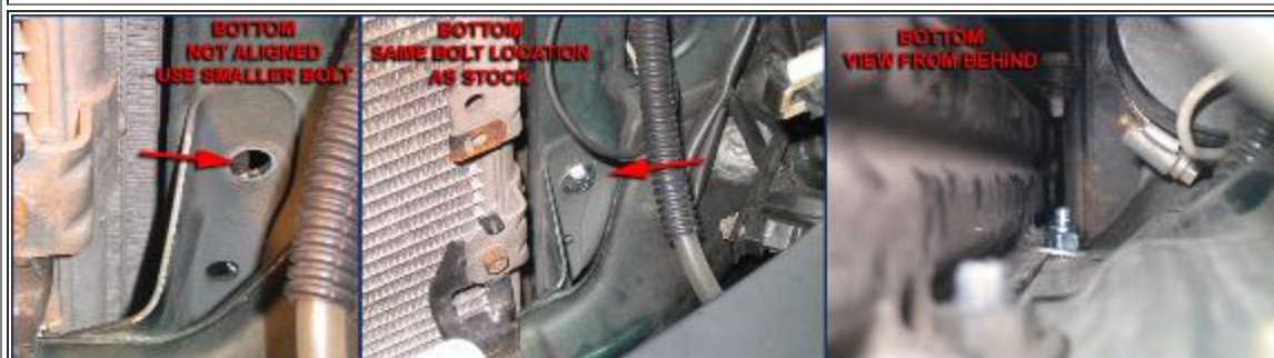
Radiator re-mounted 2" lower
