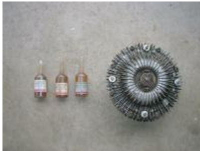
Fan clutch with silicone fluid.
