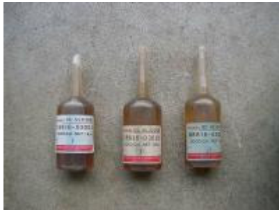
The manual says to use 50mL of 3000Cst of silicone fluid to refill the fan clutch. Each bottle is 18mL. Toyota P/N 08816-03001
