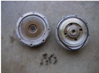
Separate the two half's and be careful not to damage the O-ring. The O-ring always seems to get stretched out.
