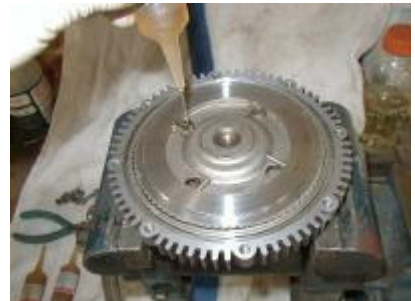
After cleaning out all of the old silicone from the fan clutch halves, add about 50mL of silicone to the lower half of the clutch. This should be just enough to fill the holes and not overflow into the O-ring groove.
